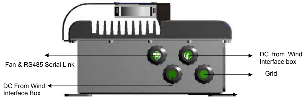
Fig.11: Position of the holes on the bottom side
